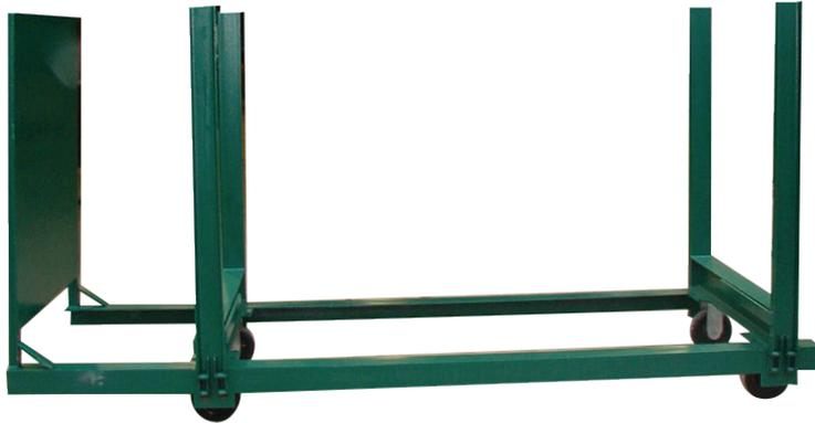
The Model 100-C is a heavy-duty one-piece lumber cart with limited pivoting uprights. The main frame is fabricated from 4" angle iron, and the uprights from 4" channel. They are equipped with 8" x 3" casters. When the bunk is full, the uprights can be released and moved slightly off 90°, allowing the pack to be lifted out with no restrictions or hang ups.
