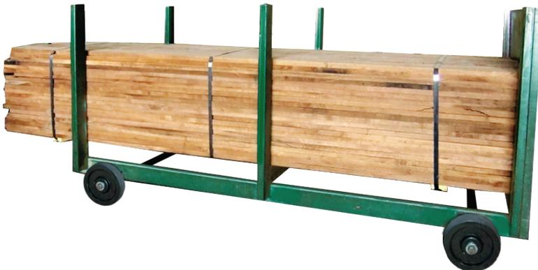
The Model 100-H is a heavy-duty one-piece lumber cart with rigid uprights. These units are fabricated with 2" x 6" structural steel tubing main rails, and the uprights are made with 2" x 4" structural steel tubing. Each cart is equipped with 12" x 3" phenolic wheels. They can be ordered in eight or ten foot lengths, or can be custom-made to your requirements.
